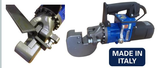
Model TP50 electric hydraulic flat bar cutter has been designed to cut maximum 50 x 16mm flat bar material with ease. This unit is powered by a reliable 230 volt / 1150 watt motor which drives the precision designed radial pump that develops a hydraulic output pressure of 570 bar, as well as an impressive cutting force of 25 Ton.
