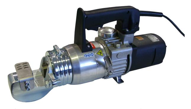
For professionals that demand the best. The T26s powerful double insulated motor drives the precision designed radial hydraulic pump which produces 32 tonnes of force. The T26 is reliable for continuous use on building sites or factory operations. Fitted with special grip to make working and carrying between jobs or worksites easier. Fitted with cutter guards for safe operation for the user.
