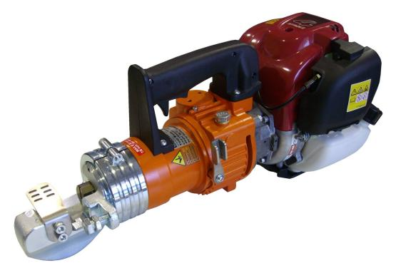
Model T22 rebar cutter - TPS22N petrol body is a cordless 22mm diameter high tensile rebar cutter. This unit is powered by a Honda 4 stroke petrol motor which drives the precision designed radial pump that develops an output of 25 tons / 570 bar of hydraulic pressure.
