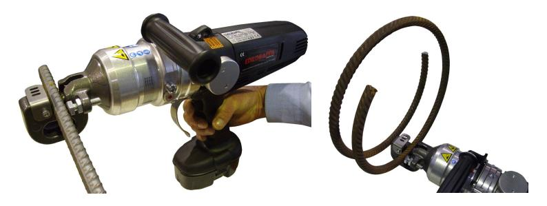
For professionals that demand the best. The Silvercut 16 cordless cutter features a powerful 18 Volt DC motor which drives the precision radial hydraulic pump which produces 12 tonnes of force. The Silvercut 16 is reliable for continuous use on building sites or factory operations. This unit is fitted with a user friendly grip to make working and carrying between jobs or worksite easier.
