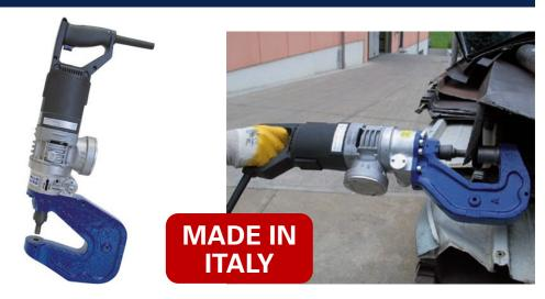
The PG22/120DE electric hydraulic hole puncher is a precision made portable puncher that can be applied to any working position in any given environment, which allows the operator more flexibility to punch holes in confined situations for a wide range of applications. The PG22/120DE can punch through 6mm (250 Grade) mild steel plate maximum thickness.
