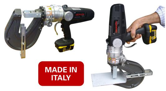
The Edilgrappa PG22 / 120 DE cordless hydraulic hole puncher is a precision made portable puncher that can be applied to any working position in any given environment, which allows the operator more flexibility to punch holes in confined situations for a wide range of applications. The PG22 / 120 DE can punch through 6mm (250 Grade) mild steel plate maximum thickness.
