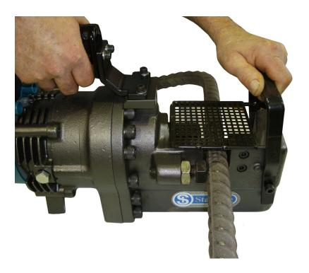
HBC-232 electric hydraulic rebar cutter have been designed for cutting maximum 32mm diameter high tensile rebar with ease for factory & on-site applications. Ogura's HBC-232 rebar cutters incorporate several safety features including an ergonomically designed cover guard system located over the moving cutter blades that provides protection to the operator when the tool is in operation.
