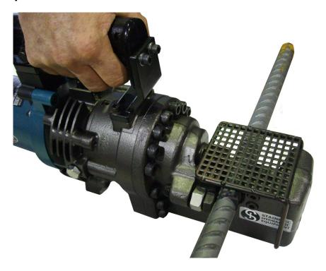
HBC-225 electric hydraulic rebar cutter have been designed for cutting maximum 25mm diameter high tensile rebar with ease for factory & on-site applications. Ogura's HBC-225 rebar cutters incorporate several safety features including an ergonomically designed cover guard system located over the moving cutter blades that provides protection to the operator when the tool is in operation.
