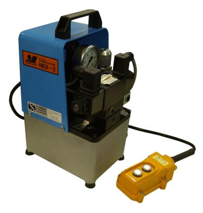
The NEX-2EGS electric hydraulic power pack pump is suitable for various applications to power small to medium sized hydraulic cylinders and tools. Being lightweight and extremely portable at 14kgs it is easy to transport between on-site and factory based operations.
