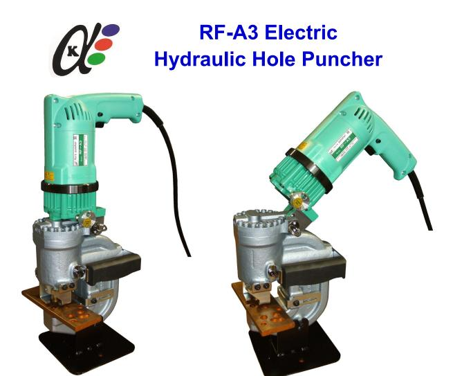
Stainelec Hydraulic Equipment has released the Kamekura RF-A3 electric/hydraulic copper bar hole puncher unit. The RF-A3 is manufactured in Japan by Kamekura Seiki. The RF-A3 hydraulic hole puncher can penetrate holes in 10mm mild steel, 6mm stainless steel, 12mm brass, 12mm copper bar and 12mm aluminium thicknesses of material. The RF-A3 punches the material with precision made punch and dies ranging from 6mm to 20mm diameter in 1mm increments.
