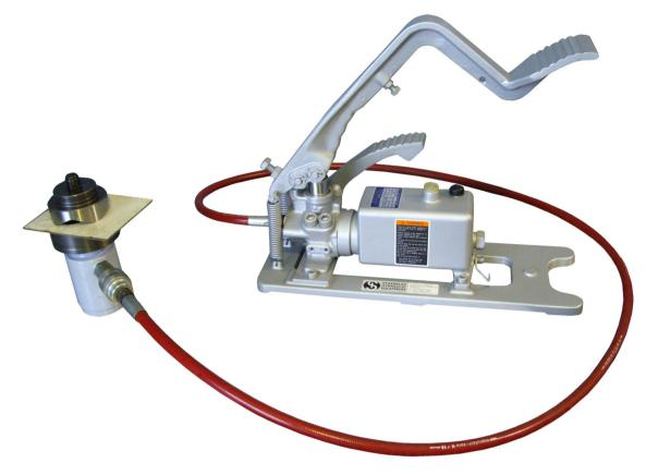
The HP-3 FPA-0.5 oil pressure foot operated pump and punching head is designed for use in punching holes in maximum 2.4mm Stainless Steel, 3.2mm Mild Steel and 6mm Aluminium plate with ease. When in use the hydraulic punching head produces a maximum punching force of up to 10 Ton and can be fitted with both round and square punching dies per customers request.
