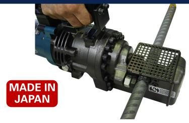
The HBC-225 electric hydraulic rebar cutter has been designed for cutting maximum 25mm diameter high tensile rebar with ease for factory & on-site applications.
