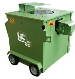
This table rebar cutter & bender is capable of cutting 32mm (650 Grade) & 30mm (850 Grade) rebar and bending 38mm (650 Grade) & 36mm (850 Grade) rebar with ease. This unit is suitable for carrying out work on construction sites where a rebar production machine is required, or for high production cutting and bending applications in fabrication workshops.
