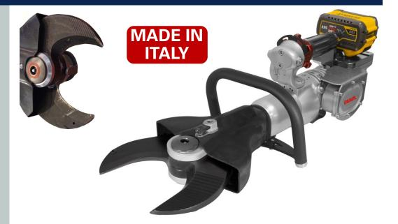
The F180-2P cordless double-acting hydraulic steel cutter is a precision engineered cutter that can be used to shear and cut through metal obstructions in extrication scenarios as well as industrial steel cutting applications. The F180-2P cutting head is hydraulically driven and can produce up to 700 Bar of hydraulic operating pressure.
