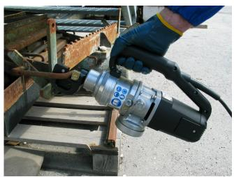
For professionals that demand the best. The Silvercut 16 features a powerful double insulated motor which drives the precision radial hydraulic pump which produces 11 tonnes of force. The Silvercut 16 is reliable for continuous use on building sites or factory operations. This unit is fitted with a user friendly top handle grip to make working and carrying between jobs or worksite easier.
