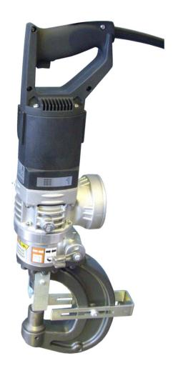
The Edilgrappa PG22/60 DE electric hydraulic hole puncher is a precision made portable puncher that can be applied to any working position in any given environment, which allows the operator more flexibility to punch holes in confined situations for a wide range of applications. The PG22/60 DE can punch through 6mm (250 Grade) mild steel plate maximum thickness.
