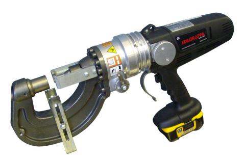
The Edilgrappa PG22/60 DE cordless hydraulic hole puncher is a precision made portable puncher that can be applied to any working position in any given environment, which allows the operator more flexibility to punch holes in confined situations for a wide range of applications. The PG22/60 DE can punch through 6mm (250 Grade) mild steel plate maximum thickness.
