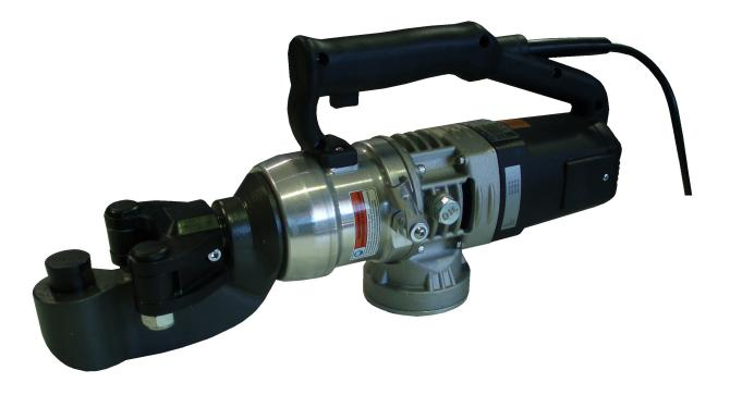
MU16P electric hydraulic rebar bender has been designed to bend 16mm high tensile rebar with ease for on-site & factory based applications. This unit is powered by a reliable 230 Volt electric motor which drives the precision designed radial pump that develops an output of 10 tons / 280 bar of hydraulic pressure.
