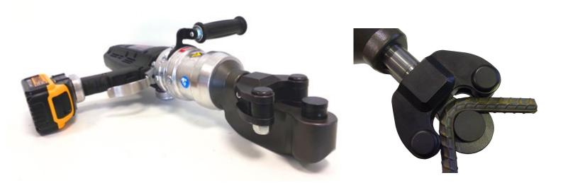
MU16P cordless hydraulic rebar bender has been designed to bend 16mm high tensile rebar with ease for on-site & factory based applications. This unit is powered by a reliable DeWalt battery motor which drives the precision designed radial pump that develops an output of 10.5 tons / 400 bar of hydraulic pressure.
