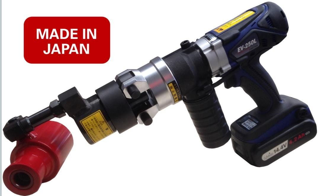
The Cactus EVK-100 Cordless Hole Punch is designed to punch through 3.2mm mild steel, 2.4mm stainless steel & 5mm aluminium material in any working position for on-site or high production applications.
