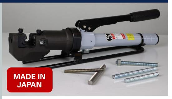
Stainelec Hydraulic Equipment introduces the DW-400 manual hydraulic threaded rod cutter. This unit gives the operator the easy task of cutting threaded rod without damaging the thread after completing the cut.
