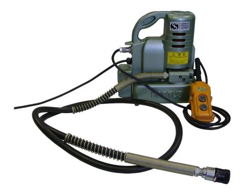
This electric hydraulic power pack pump is suitable for all applications to power small to medium size hydraulic cylinders and tools. Being lightweight at 9.5kgs and compact in design, this unit is easy to transport for site work applications. Also comes complete with standard high pressure hose.
