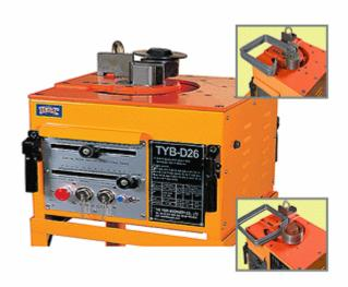
The TYB-D26 rebar bender has been designed to bend 26mm diameter rebar to a maximum bending angle of 180 degrees within 3.6 seconds. The dual angle adjustment system allows simultaneous bends for two different angles without adjusting the angle adjustment controls. The operation for each angle selection can be operated with either of the two foot switch controls.
