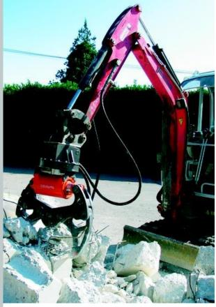
Model 430 DE T34 concrete crusher is designed to suit smaller excavators, being most useful in demolition applications were smaller excavators can be used in confined spaces with limited access.
